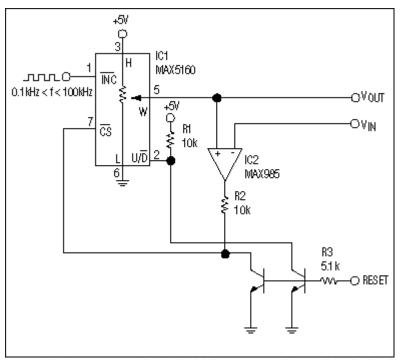
Unlike peak detectors that use a capacitor to hold the output voltage, this design includes a digital potentiometer (IC1) that holds the output level indefinitely, without droop.
